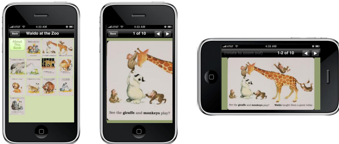
Figure 2: The overview (left), page view (middle), and rotated page view (right). Using the device’s accelerometer, the software automatically rotates the text and displays two pages in landscape mode, thus presenting a more complete view of the book.
